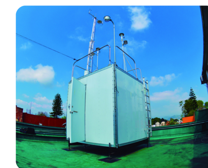
Automatic station for air quality monitoring. Image provided by Julio C. Martínez Hernández
